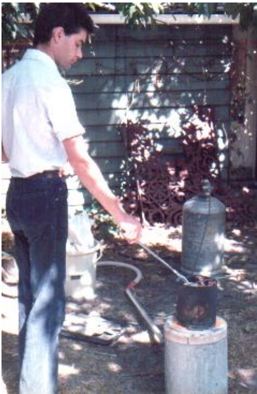
Making glass of antimony using gas and air mix blown by a reverseable vacuum cleaner for more oxygen and a higher temperature. (1200 C.)
