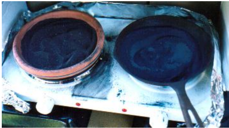
Calcination of Galena in terracotta and Antimony ore in iron frypan.
